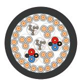
**BETA**trans® GKW flex R black UV  $3\times(6\times1,5)+1\times(4\times(2\times AWG\ 26/7)St)$  C 100 Ω GigaCAT  $7+1\times(4\times0,50)$  C 120 Ω MVB+ $2\times(2\times0,50+1\times0,50\ mm^2)$  C 120 Ω MVB
