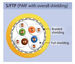
Overall braided shielding Foil shielded twisted pairs
