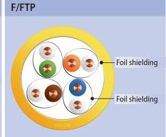
Overall foil shielding Foil shielded twisted pairs
