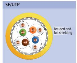
Overall braided and foil shielding Unshielded twisted pairs
